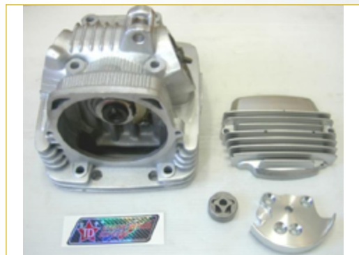
YAMAHA TW225 oversized cylinder head
