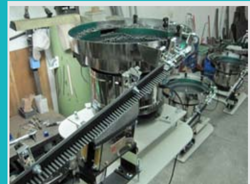
Vibrating screw feeder
