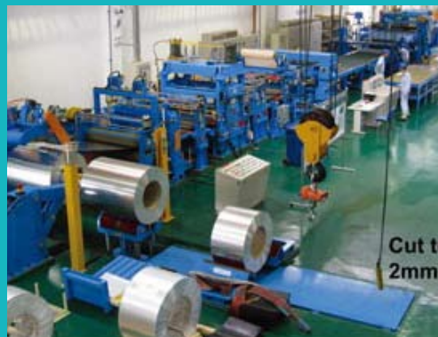
Cut to Length Line
