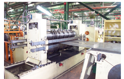
Automatic steel sheet slitting machine
