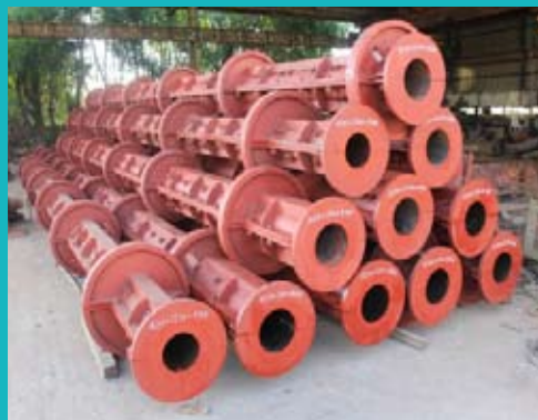
Power pole molds
