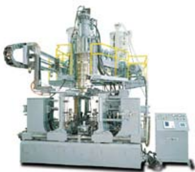
TWO-LAYER/ TWO COLOR ACCUMULATOR DIE-HEAD BLOW MOULDING MACHINE
