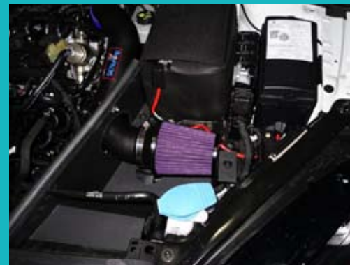
V.W. Golf 7 2.0GTI Air Intake System with heat shield
