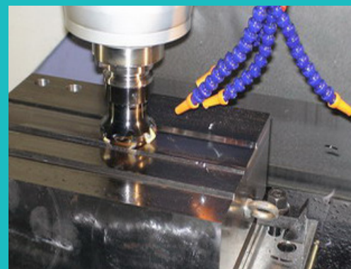
Face milling - S50C Steel
