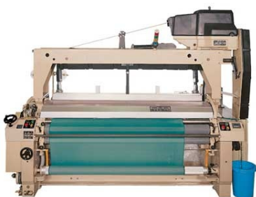
1-Nozzle Water Jet Loom with Dobby
