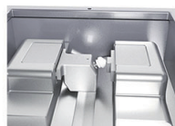
The Specimen holder for living tissue and 3D cell culture experiments.
