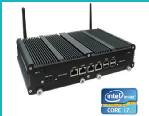
In-Vehicle Computer Intel Gen3 Core i7 CPU up to 2.8GHz with HD 4000 GPU On-Board Computer
