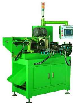
Bench Lathe(lathes both sides simultaneously)
