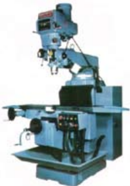
Vertical Milling Machine
