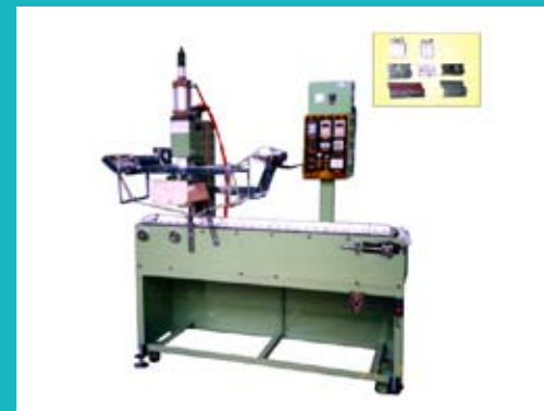
Auto-return transfer printer with pneumatic belt conveyor
