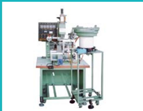
Pneumatic, automatic sphere hot-stamping machine
