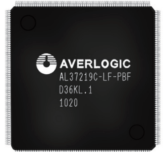
9-CH Video Surveillance Controller
