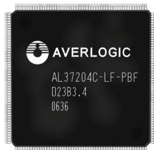
4-CH Video Surveillance Controller
