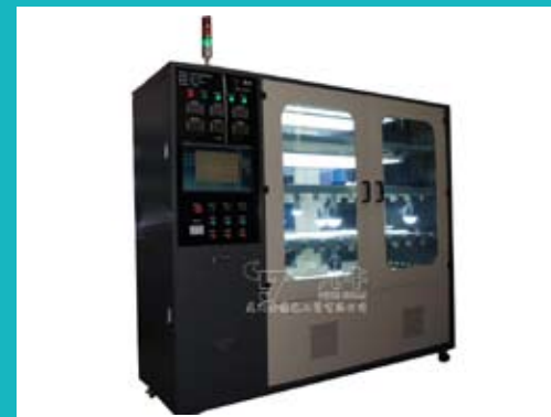
Trial LED durability testing enclosure
