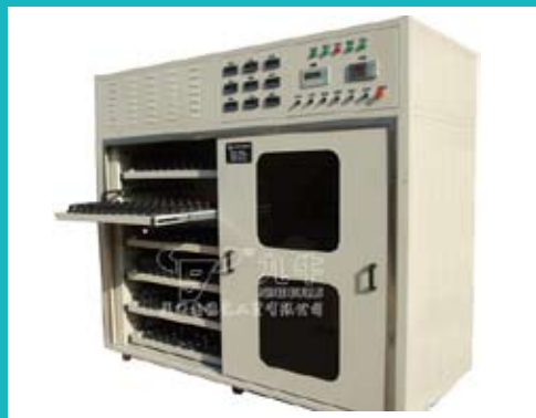
LED lighting fixture durability testing enclosure
