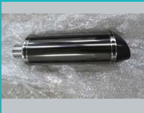
Exhaust silencing equipment
