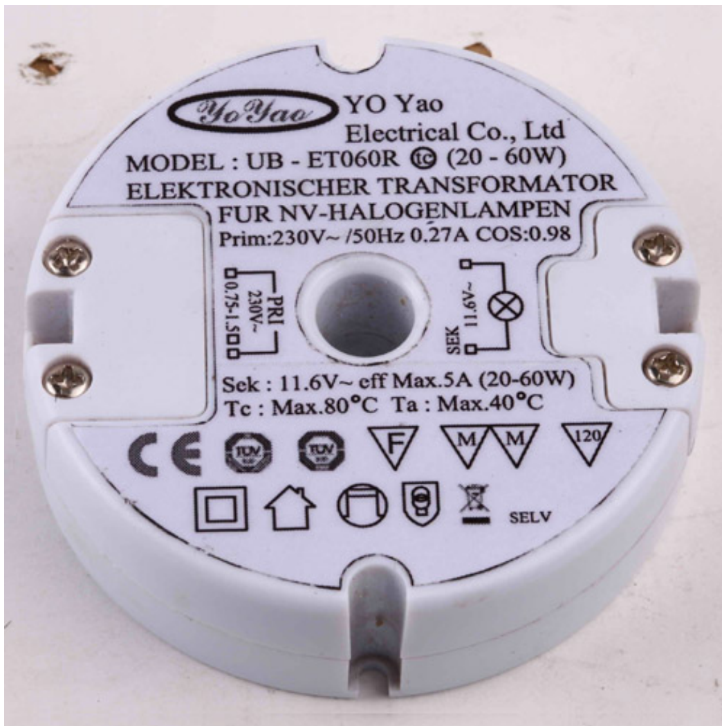
60W Electrical Transformer
